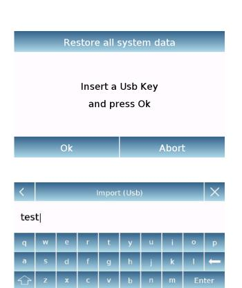
Insert the USB stick into the USB port on the left side of the device, and press the "OK" key.
