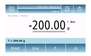
To reset the balance, remove all items from the plate and press the "- 0 -" key.
