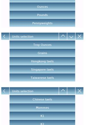
The last three units of measure, K1, K2, K3, are customizable units. For reference, refer to the chapter "Selecting the custom measurement unit".
